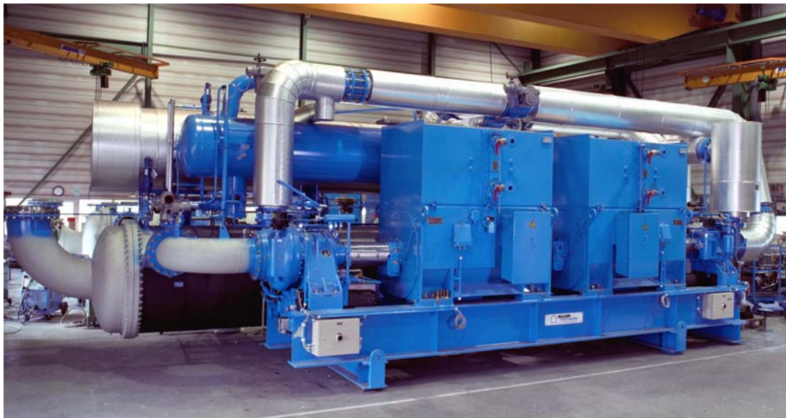
Fig. 1. centrifugal heat pump 28CPY after assembly in factory
