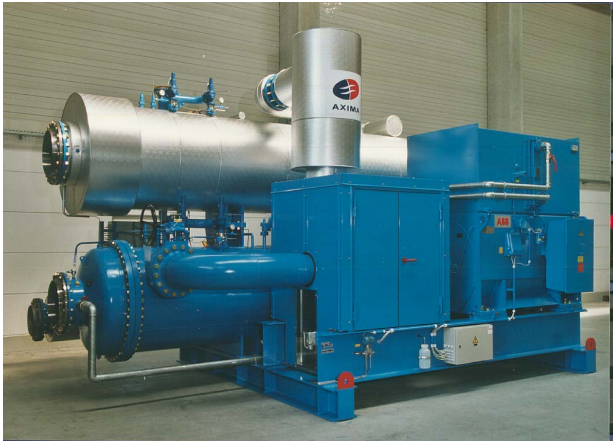
Fig. 7. Picture of the centrifugal type heat pump 28C installed at SYSAV Malmö waste burning plant (with silencing hood over the compressor)
