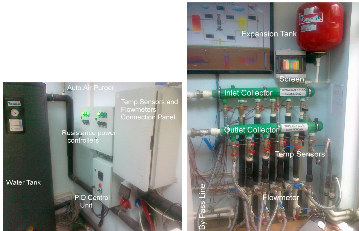
Figure 4: Thermal Response Test System Pictures
