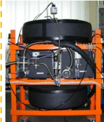
3.5 kW zeolite-water refrigerator for stationary applications
