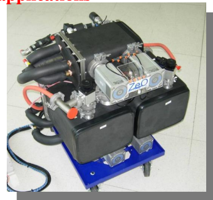
2.5 kW zeolite-water chiller for automotive applications
