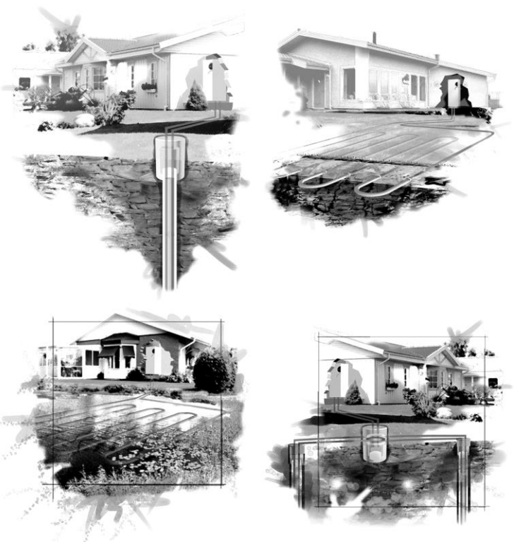
Figure 3. Collectors in rock, earth, lake and open system
