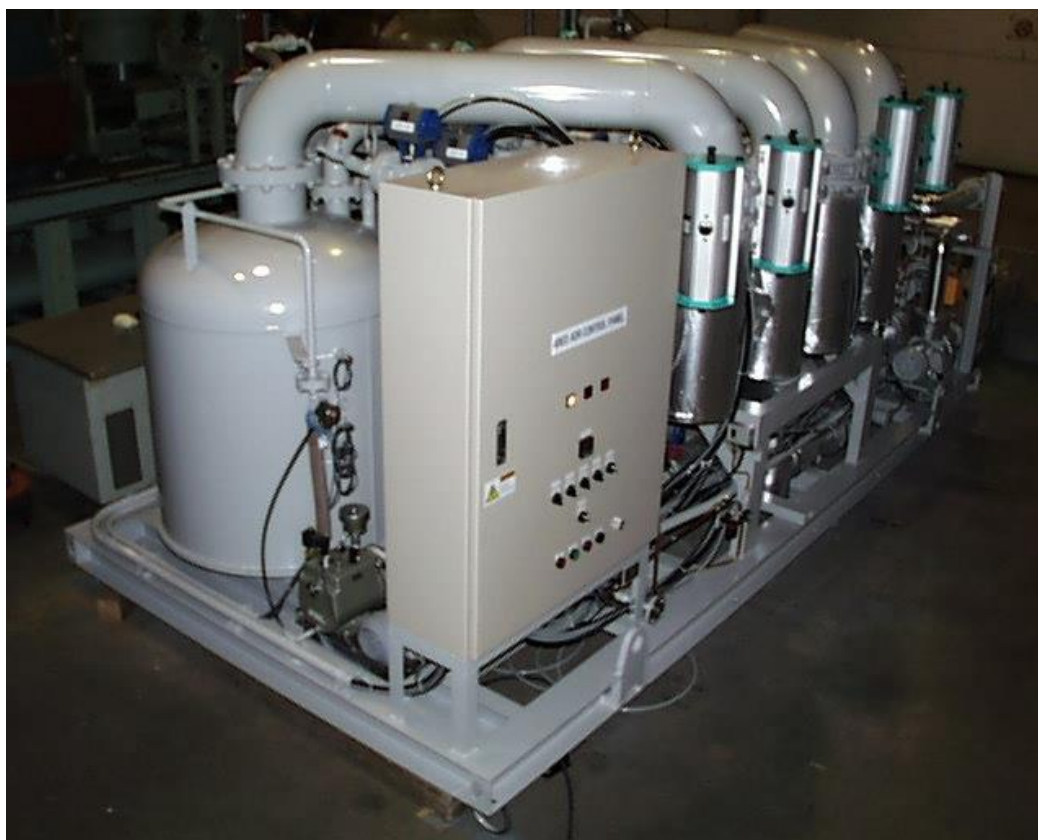
Fig.2 Set up view of the prototype 4-bed adsorption chiller with a cooling capacity of 5RT.
