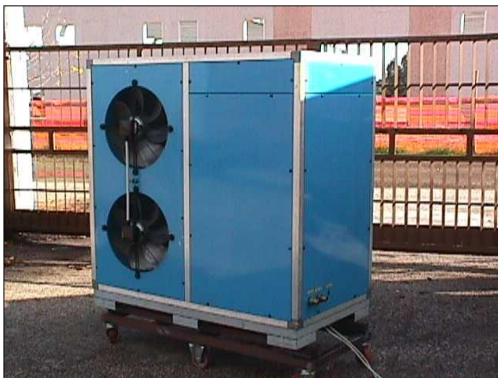
Photo 2. The 11 kW Machine - Dimensions: 85 x 155 x155 cm
