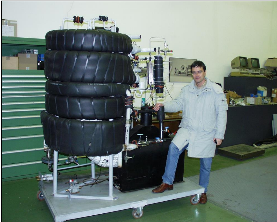
Photo3. The 25 kW Machine (lab. prototype) - Dimensions: 100x180x200 cm
