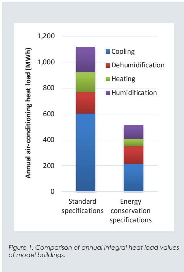
Figure 1. Comparison of annual integral heat load values of model buildings.
