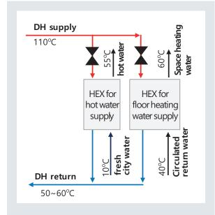
Fig. 1: Schematics of conventional Korean DH system and temperature conditions for an apartment complex in winter.
