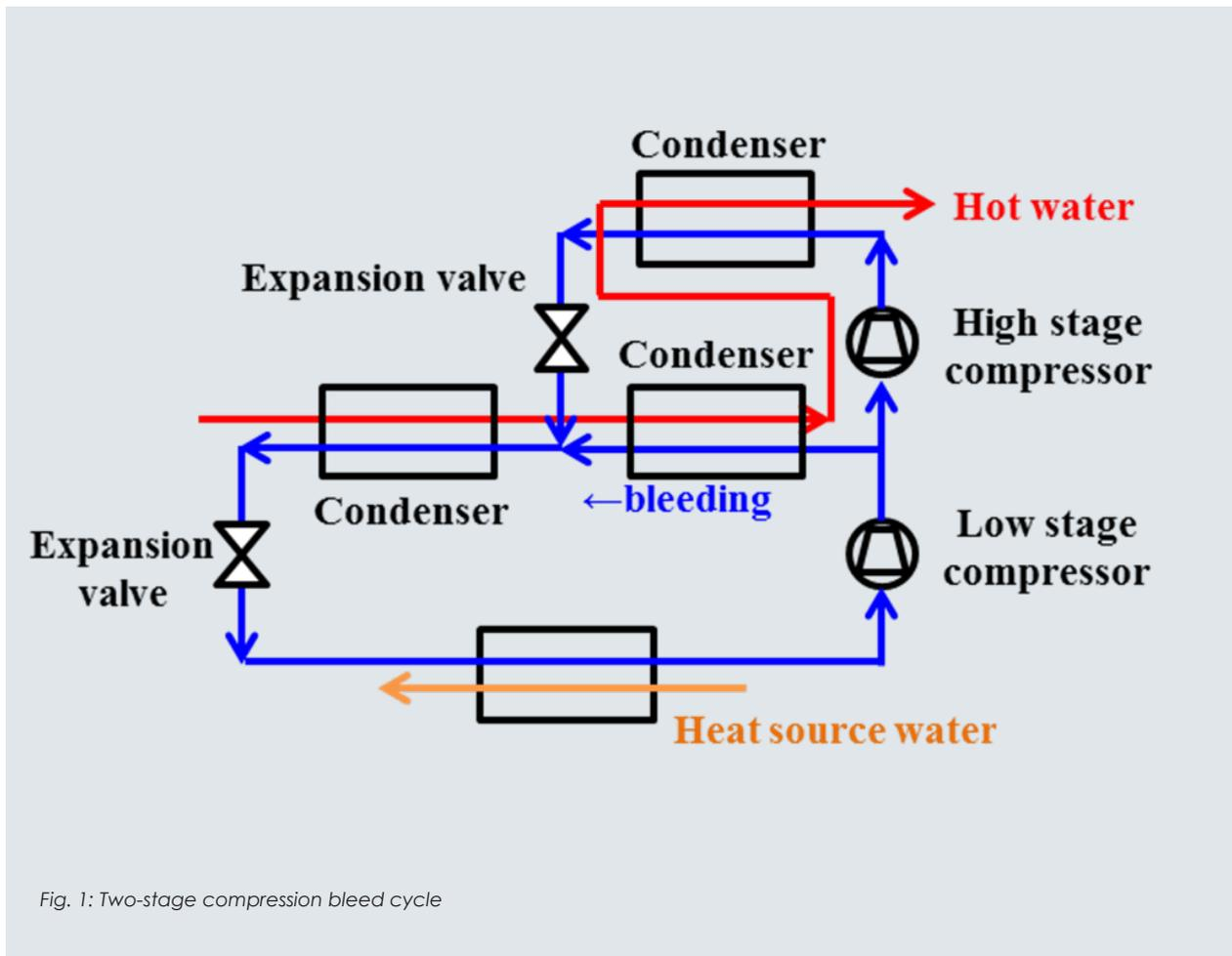
Fig. 1: Two-stage compression bleed cycle
