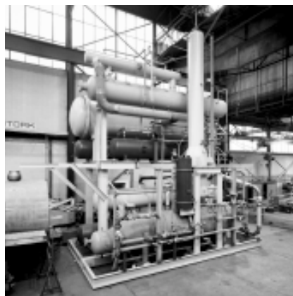
▼ Photo 2: A steam-driven absorption refrigeration system.
