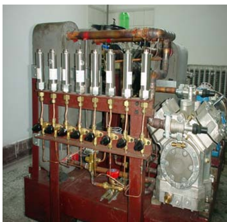
Figure 1: Test stand of heat pump driven by bi-fuel engine
