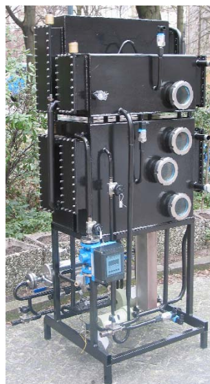
Figure 1. Prototype of the 10 kW absorption chiller and technical data
