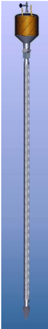
Fig. 12. FKW Heat Pipe
