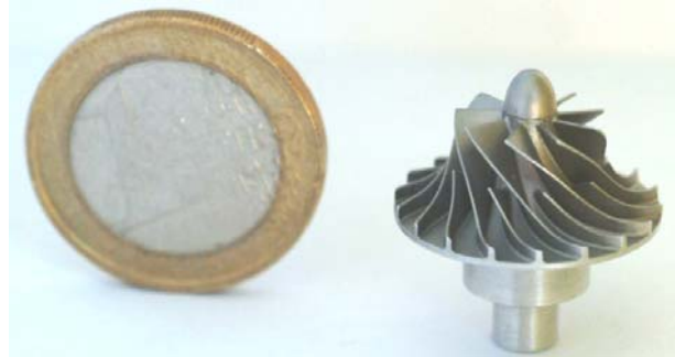
Fig. 5. The machined compressor wheel in comparison with a 1Euro coin.
