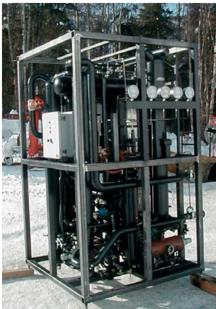
Figure 2. Double lift ThermoChiller prior to installation
