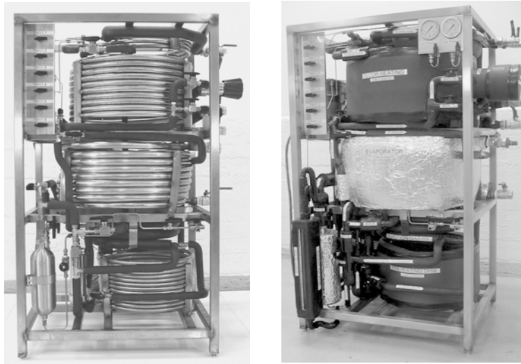
Fig. 3. The prototype CO 2 heat pump unit for combined space heating and hot water heating.
