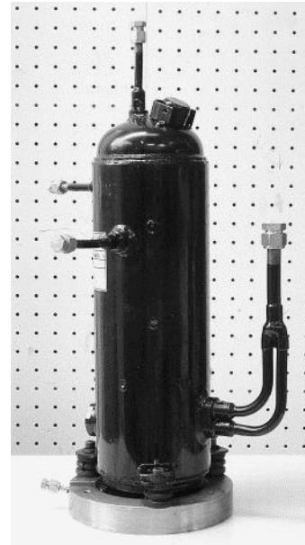
Fig. 3 Structure of hermetic prototype of Expander-Compressor Unit
