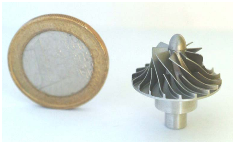
Fig. 4. Turbocompressor for R134a compared with a Euro coin.
