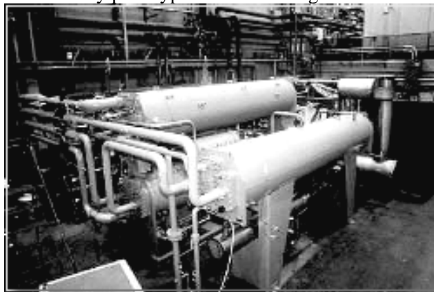
Fig. 3. Trane's Laboratory Prototype Dual-Loop Triple-Effect Chiller
