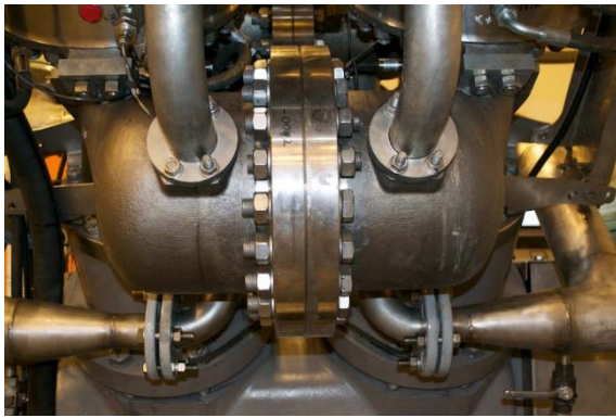
(a) Heat exchanger package: cold side on the left and the hot side on the right. Water inlets and outlets are respectively on the bottom and top side for both hot and cold side.
