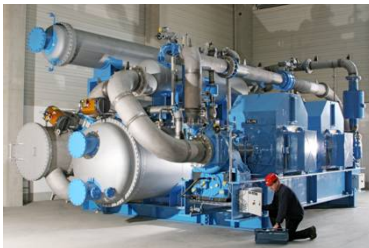
Figure 2: The 3 rd Sandvika heat pump UNITOP 33/28 in FRIOTHERM workshop.
