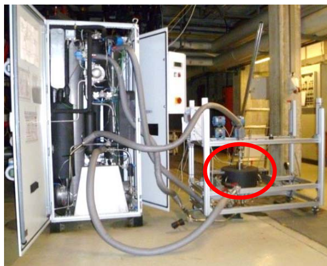
Figure 8: Picture of the ThermoPump test bench (PinkChillerPC19) with the prototype of the Thermo-Pump (red circle) (Zotter & Rieberer 2013)
