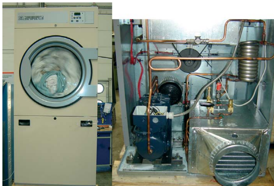
Figure 4: Heat pump in commercial clothes drier (front and back)
