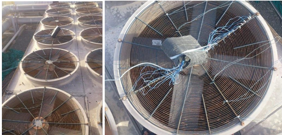
Figure 6: Condenser Fan Thermopile and Thermocouple Rake Installation
