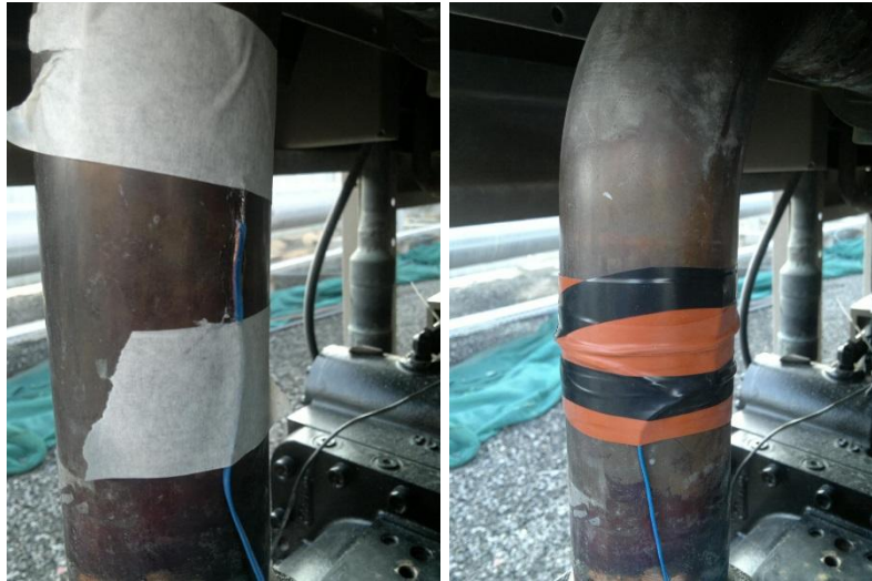
Figure 4: Thermocouples Surface Installation
