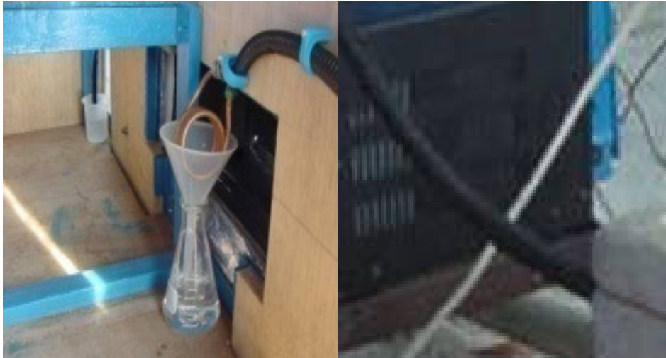
Figure 3. Improvised actual moisture content meter
