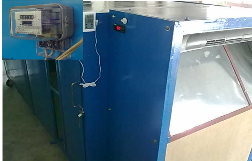
Figure 5. Watt-hour meter installed outside the drying chamber
