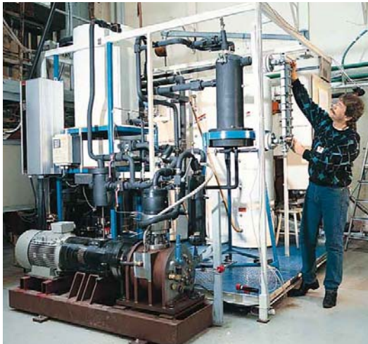
Fig. 5. 50-kW prototype heat pump water heater in SINTEF/NTNU laboratory
