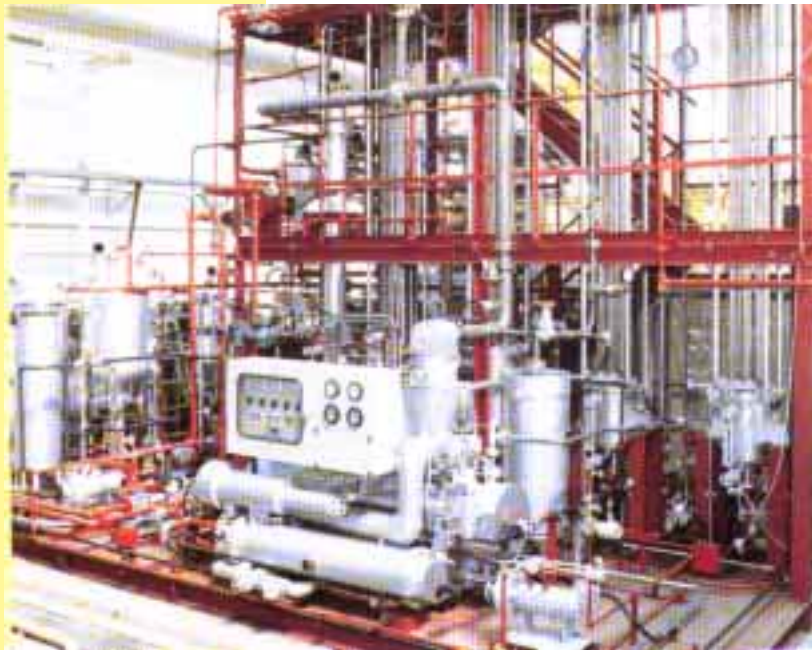
Above: Innovations are leading to high-temperature IHP applications. This Japanese prototype delivers heat at 200°C.
