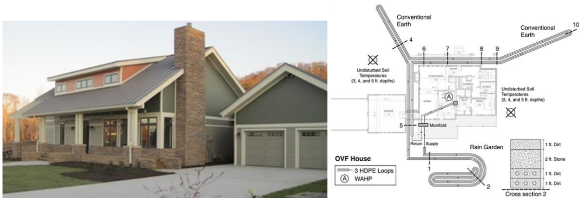
Fig. A 2: Test site (left) and GHX layout (right)
