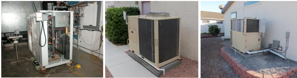
Fig. 42: Development steps of the Gas-engine AS-IHP: Alpha (1 st generation) prototype – lab test set up (left), Alpha prototype at field test site in Las Vegas area (middle) and Beta prototype field test unit (right).
