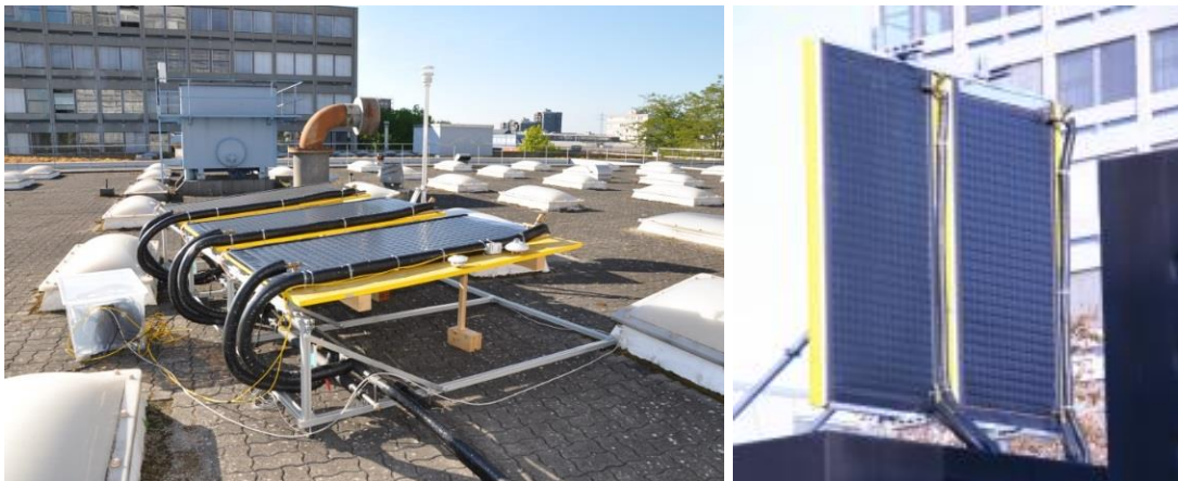
Fig. 25: Installed absorbers on the roof of the Energy Research Lab
