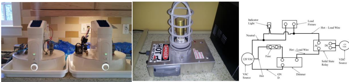
Fig. 51: Latent load generators (left) and sensible load generators (right) of the occupancy emulation installed in the NZERTF
