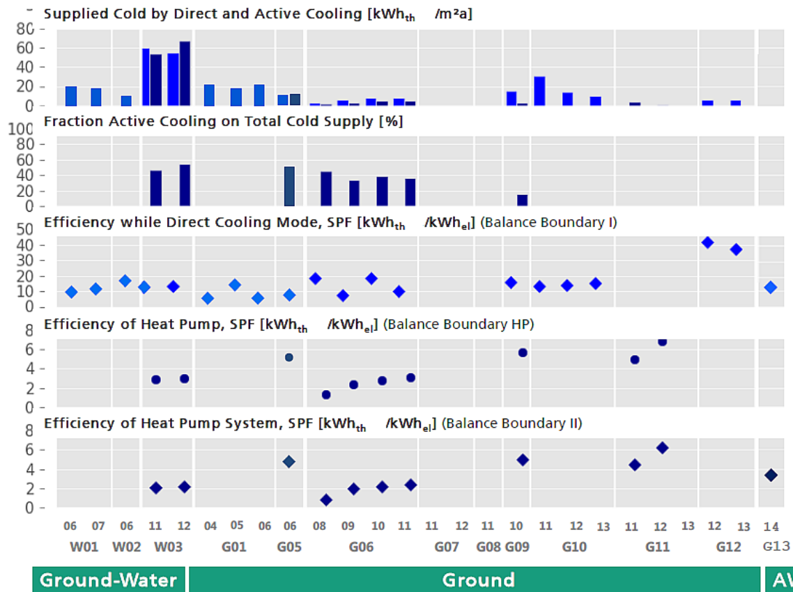
Fig. 15: Evaluation of cooling energy and fraction of active cooling as well as SPF according to boundary I, HP and II for the analysed systems
