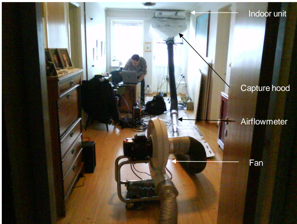
Figure 4. Measurement equipment due to SP Method no. 1721
