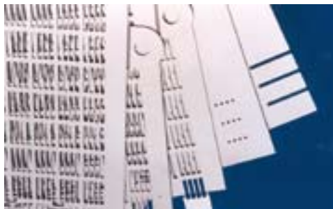
The photo shows a compact heat transfer surface, in the form of a 'shim' used in heat exchangers produced by Chart Energy & Chemicals, Inc.
