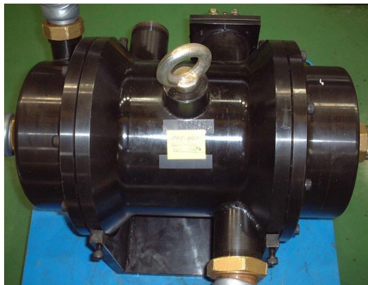
Figure 2. Two stage variable speed centrifugal compressor
