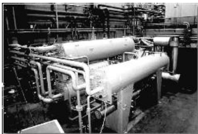
Figure 3. Trane's Laboratory Prototype Dual-Loop Triple-Effect Chiller.
