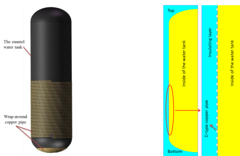
Fig. 1. Schematic diagram of 3D model structure of water tank Fig. 2. Schematic diagram of 2D model structure of water tank
