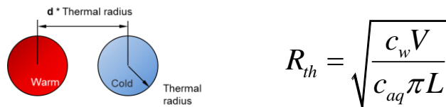
Figure 5. ATES well layout and footprint definition. Thermal radius depends on thermal properties of aquifer and water ( c_{aq} , c_w ), storage volume ( V ) and filter screen length ( L )
