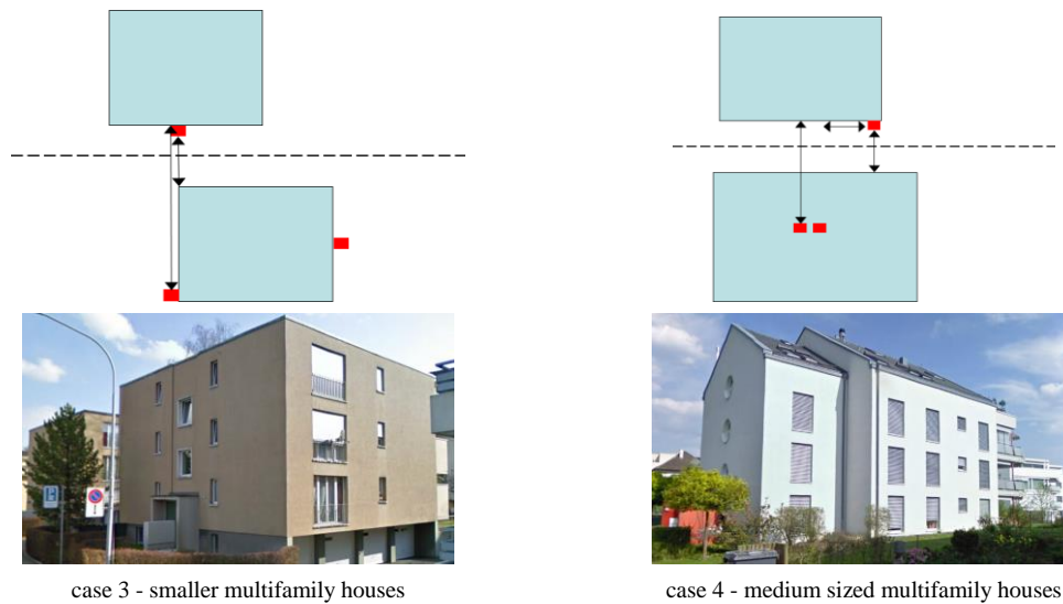
Fig. 8. Case sketch with indicated land boundary (-----), possible heat pump location / sound source ■, distance between sound emission point and place of impact ↔
