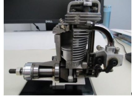
Cut model of engine
