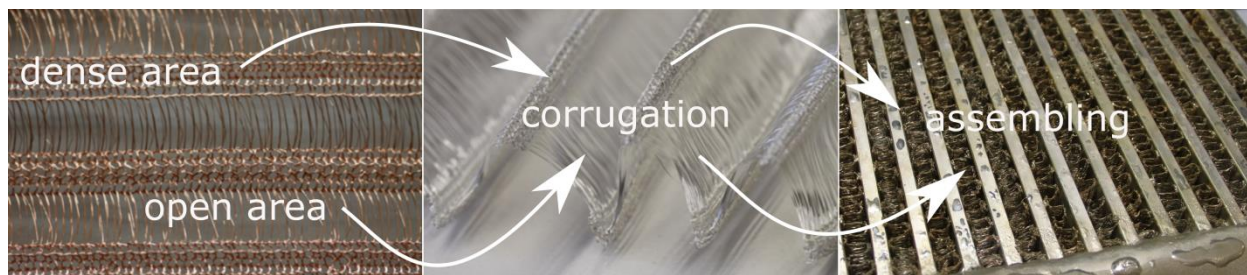
Fig. 2. Possible manufacturing process steps of wire structure heat exchanger: A knitted fabric with dense and open areas (left) is corrugated in first process step to a 3D structure (middle). In second process step dense areas are contacted to flat tubes, open areas fill space between flat tubes (right).
