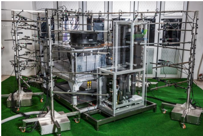
Fig. 1. Demo-Setup of the 64 microphone “acoustic dome” positioned around the GreenHP . This measuring dome allows for a flexible positioning of the microphones in different distances as all six stands can be changed in height and arranged in varying number and position to each other.
