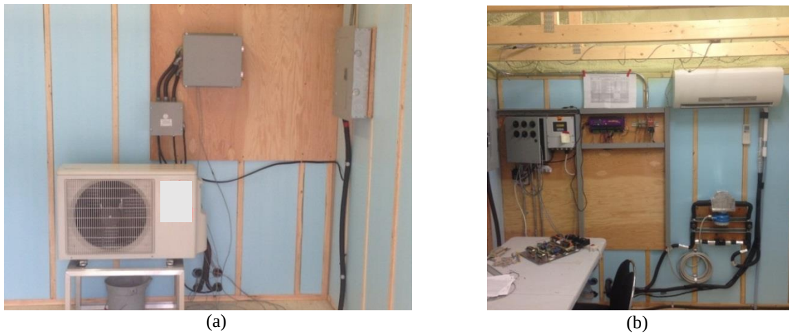
Fig. 6. Fully Instrumented (a) Outdoor Unit and (b) Indoor Unit
