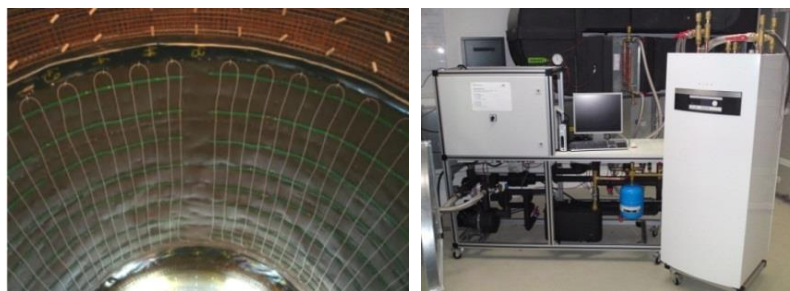
Fig. 1. Left: Tunnel section with absorber pipes before completion of tunnel lining, Right: Test rig inside control room
