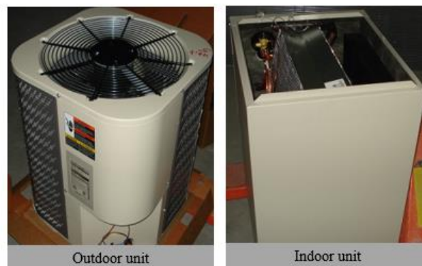
Fig. 1. Pictures of the indoor unit and outdoor unit for the 3Ton unitary split heat pump system.
