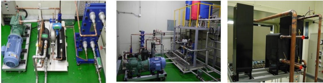
Figure 5 Experimental apparatus of steam generation heat pump development
