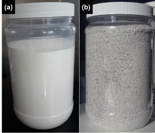
Fig. 5. Pictures of (a) powder-form and (b) granulized form of the synthesized adsorbent.
