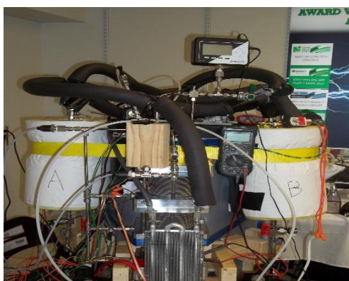
Figure 12: 50-gal Hybrid Hot Water Heater Test Prototype
