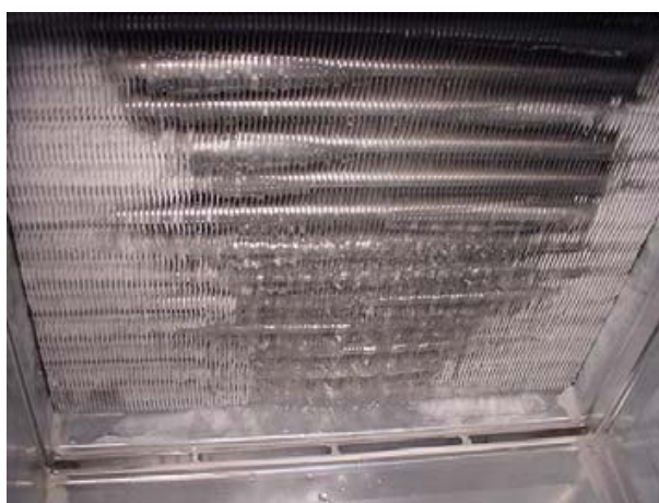
Figure 65: Fin heat exchanger at the air outlet side with partial ice accumulation (Berlinger 2008)
