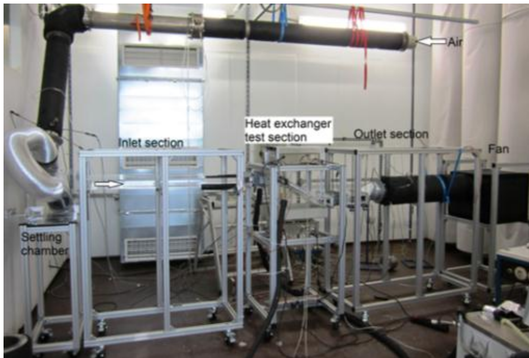
Figure ES-6: Small-scale wind tunnel at AIT (Zottl, 2016)
