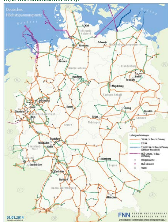
Figure 8 – German electricity transmission network: 380 kW (orange), 220 kW (green), 150 kV (blue), HVDC (purple); for each type: solid line (existing), dashed line (in process of construction), dotted line (in process of planning). Source: [2014 VDE Verband der Elektrotechnik Elektronik Informationstechnik e.V.].
