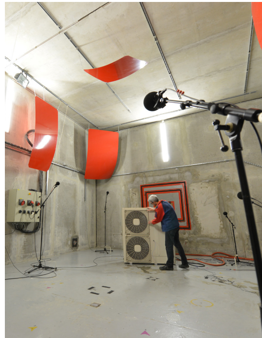
Figure 1. Outdoor HP unit installed in CETIAT's double reverberant room.
