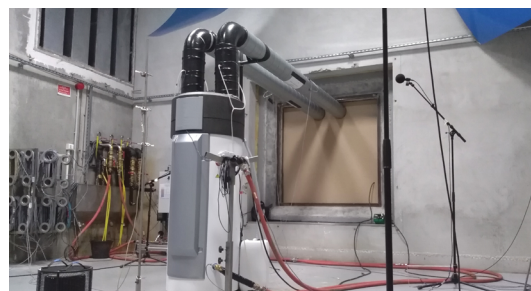
Figure 5. Exhaust Air Heat Pump Water Heater unit installed in CETIAT's double reverberant room.
